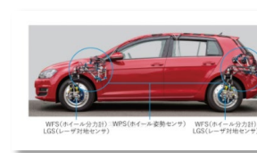
Vehicle-mounted integrated Measurement System (VMS)
